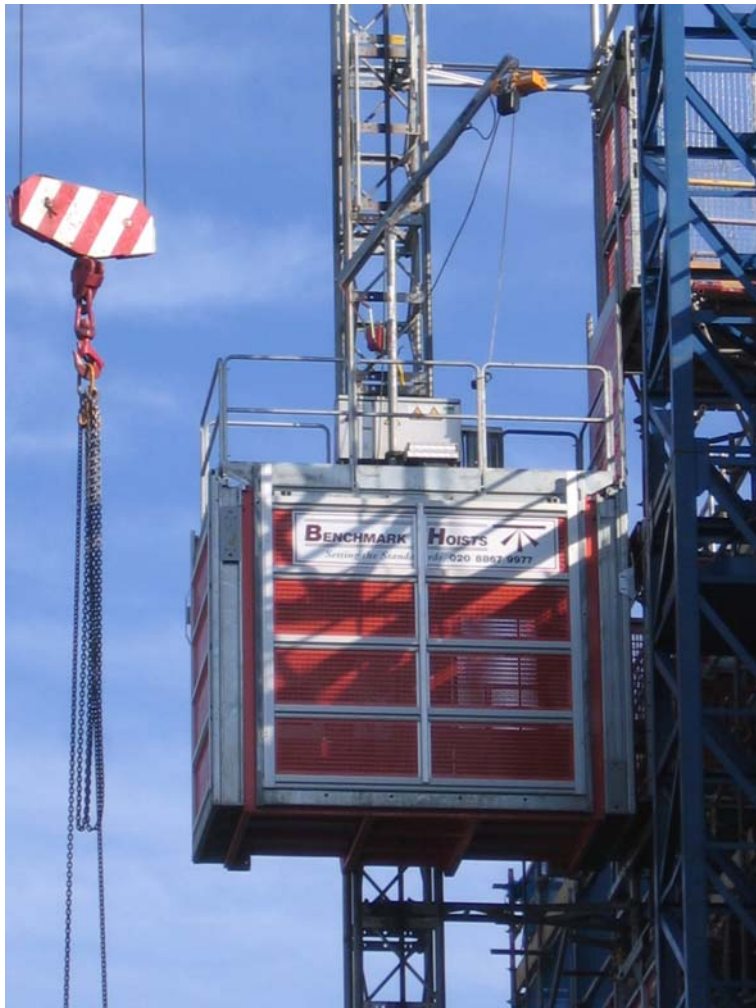
Photo 2 - Alimak 650 23/32 - shows C door 2.5m wide in side of cage for side loading at base level
